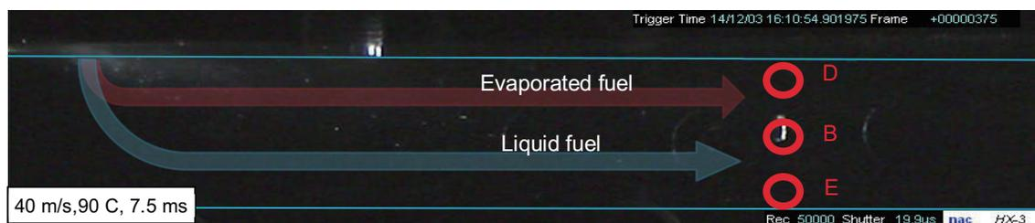
Fig.20 Passages of evaporated fuel and liquid fuel
