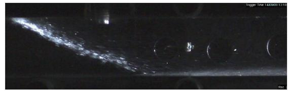
Fig.16 Spray picture (n-heptane, 40 m/s, 60 C, 7.5 ms)
