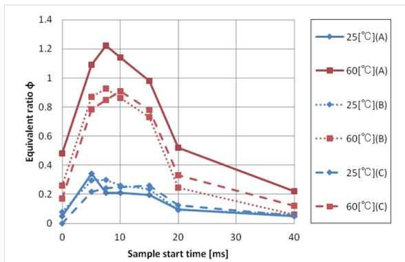
Fig.14 Equivalent ratio (n-heptane, 60 C)
