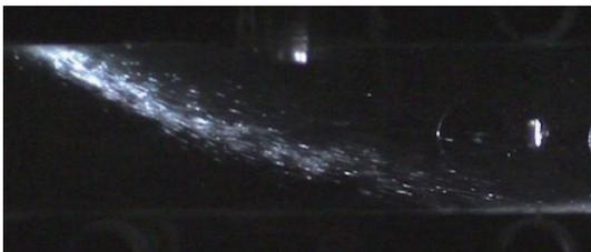
Fig.24 Spray picture (n-heptane, 40 m/s, 90 C, 7.5 ms)
