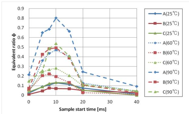
Fig.6 Equivalent ratio (n-heptane, 40 m/s)
