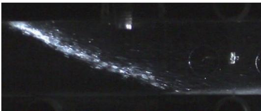
Fig.23 Spray picture (n-heptane, 40 m/s, 60 C, 7.5 ms)
