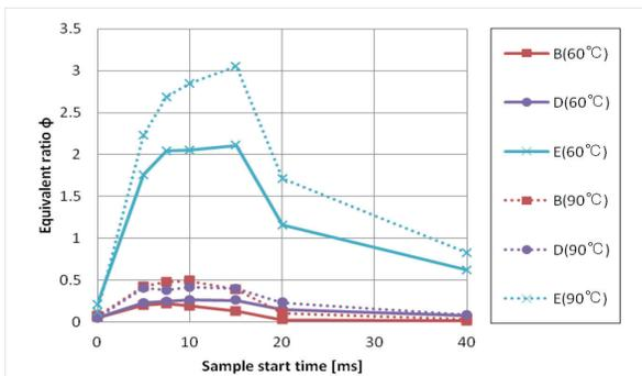
Fig.7 Equivalent ratio (n-heptane, 40 m/s)
