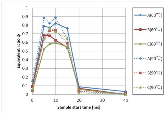
Fig.9 Equivalent ratio (i-pentane, 40 m/s)
